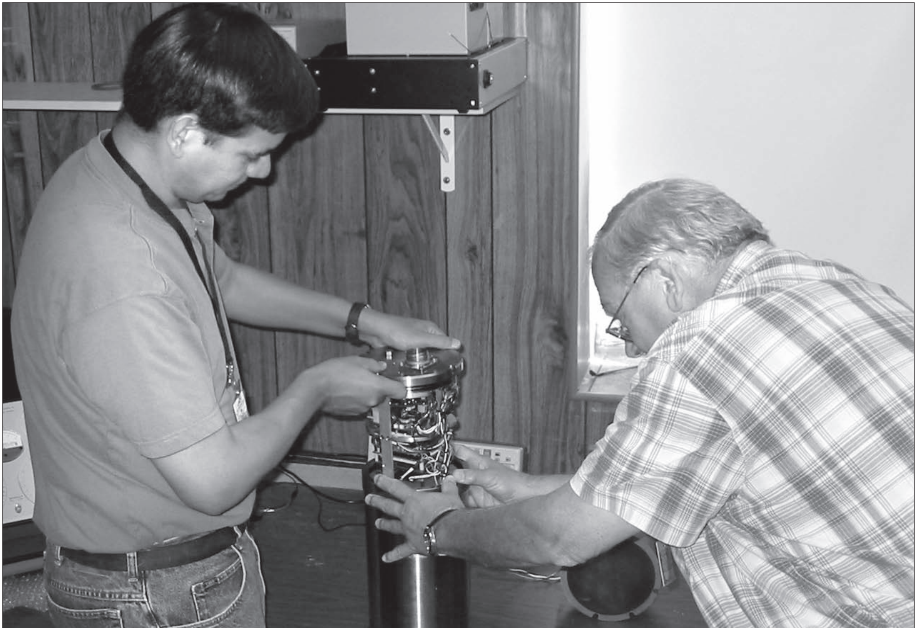
Omni Technologies engineers John Bradley and Francis Grosz examine the main electronics assembly of the company's sub-bottom profiler that examines what's underneath the seafloor.
